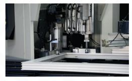
11 pieces of profile cleaning blade and two independed cleaning unit, cleaning bottom, top, interior and external surfaces of the profile.
