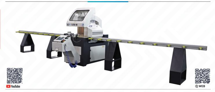
LEO-X, automatic Radial Saw with 2 axis servo controlled and 550 mm saw is ideal for cutting aluminum and PVC profiles with different angles and thickness. LEO-X designed for cutting wider profiles with the servo motion system, automatic positioning at all degrees between 90° and 30° allows for perfect cutting operation. Safety is a topmost priority for LEO-X together with the horizontal clamps and the vertical clamp along with profile protective shield which improve the cutting quality.
