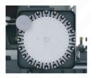
High speed rates on axes and internal automatic tool replacement magazine which moves with gantry for 20 tools allow for time savings when running different processes which require tool replacement.
