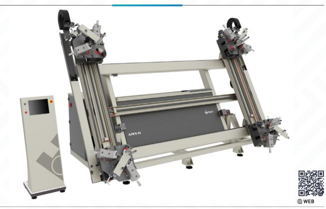
APEX - IV features simultaneous assembling of all 4 corners of the profile by combining the precision of servo positioning and power of hydraulic system to offer quick solutions to users. APEX - IV enables a seamless corner assembling process by minimizing user errors thanks to the two-stage hydraulic pressure system.
