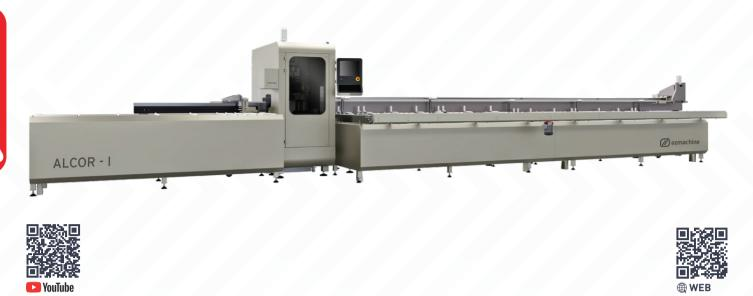
The 5 servo axis CNC profile cutting center ALCOR - I is designed to cut profiles made of aluminum, PVC and all kinds of light alloy profiles. The cutting unit with a 550 mm diameter saw blade for cutting at every angle between 30° and 150° offers a wide cutting range to users. Thanks to the feeding capacity of 10 profiles, the conveyor structure enables batch processing, letting the machine to be used in the most efficient manner.
