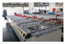
Conveyor with 4 profile feeding capacity ensures the machine to work in the most efficient way.
