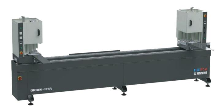
**ORION - II SN** which is automatic double head zero-normal PVC welding machine, is used for welding processes in various perspectives of plastic profiles. It can weld between  $60^{\circ}$  and  $180^{\circ}$  in one head. Through welding time, digital controlled heat and electronic thermostat, it enables to its users to weld between heat values of  $0^{\circ}\text{C}$  -  $350^{\circ}\text{C}$
