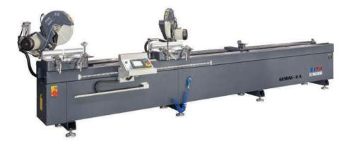
Semi-automatic double head saw with 400 mm saw blades **GEMINI – II A** is ideal for cutting aluminum, PVC and wood profiles in various angles and thickness.
