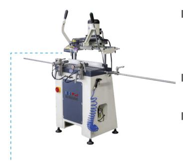
Used for cutting appropriate slots on aluminum and plastic profiles for mounting locks, grips, hinges, latches and opening channels.
