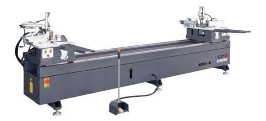
**APEX - II**, which has automatic hydraulic double head corner crimping, is used for corner binding processes for aluminium profiles. Incorporating manual metering precision and the power of hydraulic system in its body, it provides its users with quick solutions.
