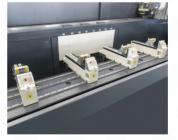
The GARNET XS, which positions its clamps fully automatically using the X-axis, completely takes on the user's workload.
