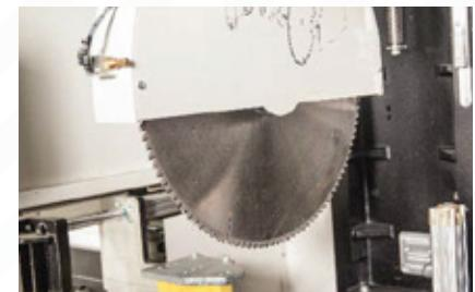
Unlock a vast array of cutting possibilities with the unit's 550mm diameter saw blade, capable of tackling any angle between 30° and 150°. This expansive cutting range empowers users to maximize their creative and production potential.
