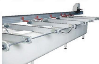
Equipped with a 10-profile feed conveyor, ALCOR - II R leverages batch processing technology for enhanced operational efficiency
