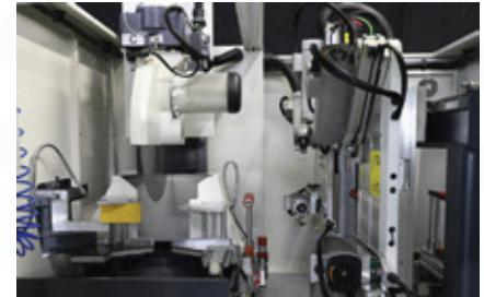
The cutting unit with a 550 mm diameter saw blade for cutting at every angle between 30° and 150° offers a wide cutting range to users.
