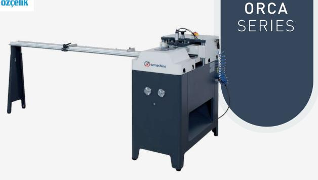
The ORCA family of rising blade saws tackles vinyl window strip cutting at a precise 45° angle with effortless ease. The pneumatic cutting system ensures clean and efficient cuts, while the automatic return to the starting point minimizes downtime.
