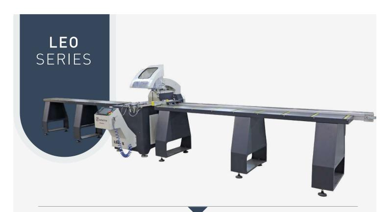
The LEO family of single head front blade saws tackles aluminum, pvc profiles with effortless ease, thanks to powerful hydro-pneumatic cutting servo-controlled rotation axis. Prioritize safety with the secure cutting cover and safety sensor, while enjoying automatic positioning from -22,5° to +45° via the intuitive servo motion system.
