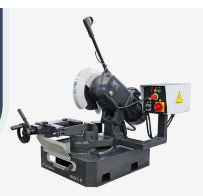
The HEKA single-head saw family is designed for cutting support plates and profile tubes. The double spring and saw guard ensure smooth, precise, and safe cutting. Manual horizontal clamps hold your profiles securely during cutting.
