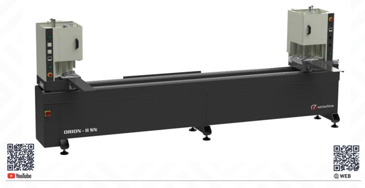
ORION - II SN which is automatic double head zero-normal PVC welding machine, is used for welding processes in various perspectives of plastic profiles. It can weld between 60° and 180° in one head. Through welding time, digital controlled heat and electronic thermostat, it enables to its users to weld between heat values of 0°C - 350°C
