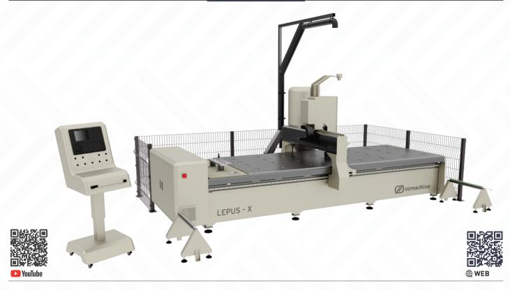
The 3-Axis CNC controlled panel and profile processing machine LEPUS - X is developed to cut v - channel opening and similar operations on various composite panels and plates. Thanks to its automatic tool magazine system with capacity for 5 tools, LEPUS -X saves time when switching to different operations. In addition, LEPUS X enables processing of aluminum, wooden, plastic and various materials by replacement of the milling cutter.
