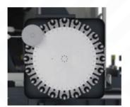
High speed rates on axes and internal automatic tool replacement magazine which moves with gantry for 20+1 tools allow for time savings when running different processes which require tool replacement.
